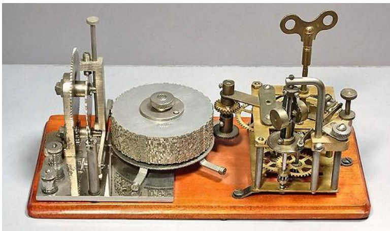
Figure 31: Omnigraph - used by FCC examiners to give morse code examinations during the 1910s and 1920s.
